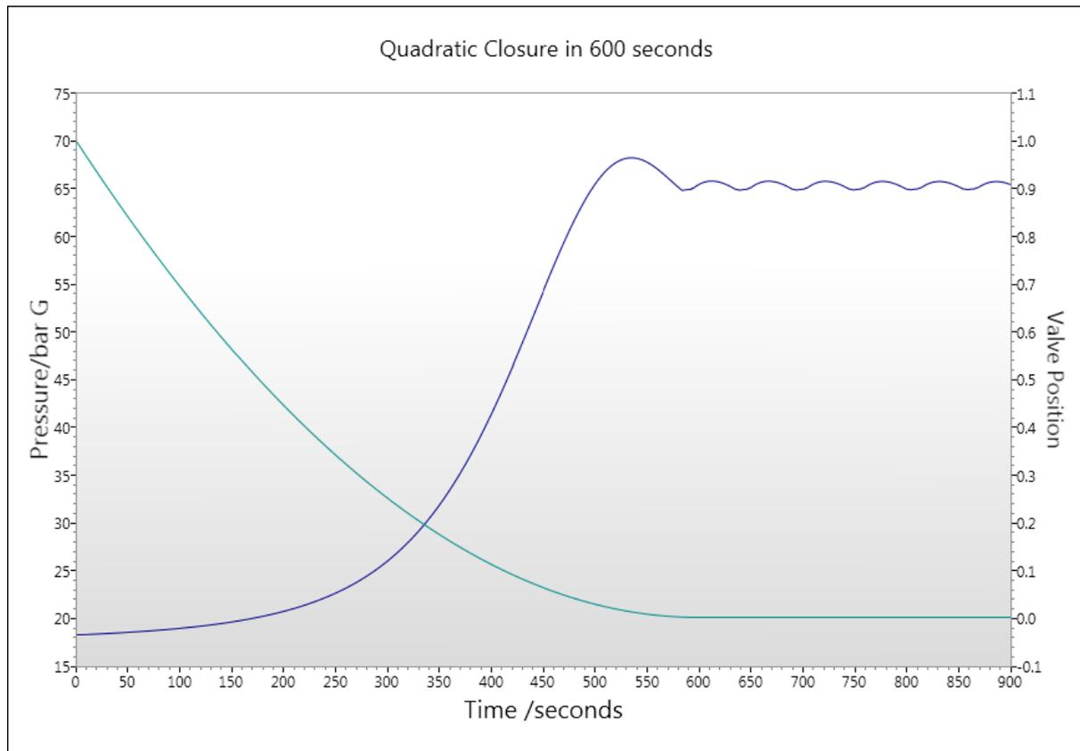
The effect is to reduce the maximum pressure at the lowest point of the system to 68 barg. It is difficult to reduce this significantly. The closed head of the pump is 57 bar. The additional pressure due to static head is approximately 7 barg. The pressure at the lowest point would therefore be 64 barg even without any pressure surge.
