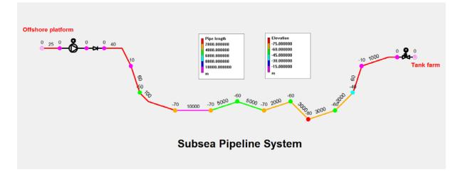
Pipes have been colour coded to show length, and nodes have been colour coded to show elevation.
