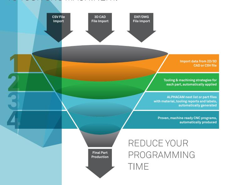
Using a conventional CAM system each file would have to be processed individually by inserting the file, extracting the features, applying tool directions and toolpaths, saving the file and NC code, and then generating the required reports. ALPHACAM can do this repetitive labour intensive work automatically.
